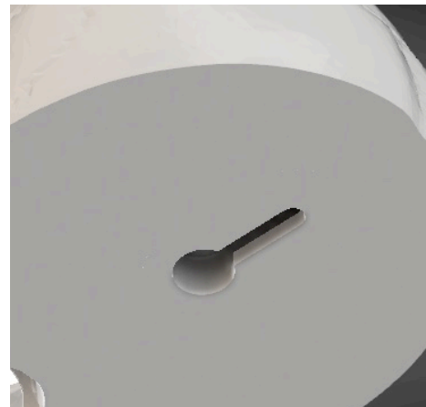
Fig 3. Hanger closeup. Own work. Rendered in Fusion 360.
